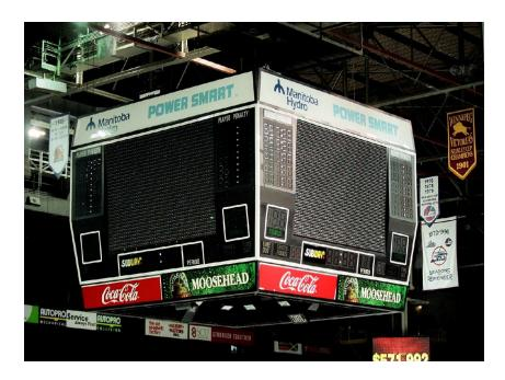
The clock was purchased new from Whiteway Sign in 1985. It measures approximately 24' x 24' x 20'h. Its approximate weight is 25,000 lbs. It contains an incandescent matrix display that measures approximately 16'w x 12'h on all four (4) sides. A Whiteway Sign operating program with a QNX operating system that controls the matrix. Included in the sale is a 5-8 year supply stock of replacement bulbs for the matrix display.
